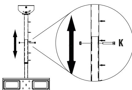
**EN:** Secure the length of the console support rod as desired using the screw (**K**) in the box.
