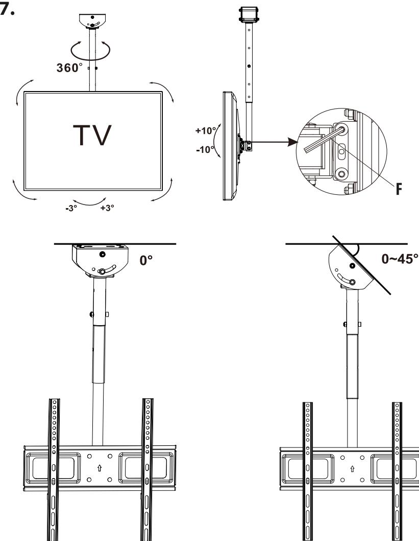
**EN:** You can adjust the angle of the TV by loosening and fixing the two allen screws on the back. The device can be rotated 360° after correct mounting. The manufacturer and distributor shall not be liable for any damage resulting from improper mounting.
