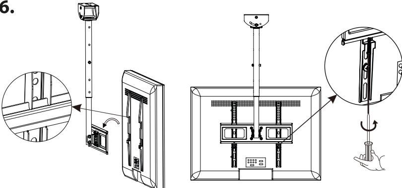
**EN:** If you have verified that both the rail and the bracket are securely fastened to the ceiling, ask for help in mounting and securing the unit. You can secure it using the two star screws on the bottom of the console.
