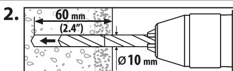
**EN:** Drill 6 holes according to the markings in which to insert the anchors marked with the letter **(I)** (10 x 50). Use a drill bit 10 for the operation, the depth of the hole should be 60 mm!
