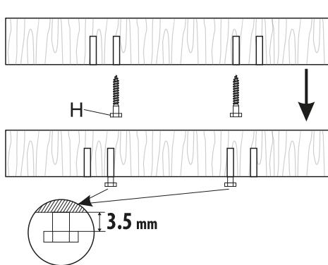
**EN:** Try the M8 x 60 screws marked **(H)** in the anchor in the hole. There can be a maximum distance of 3.5 mm between the plane of the ceiling and the screw head so that you can properly secure the bracket head.
