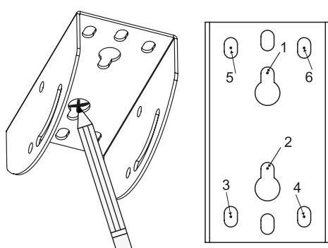
**EN:** After selecting the appropriate load-bearing location for mounting the bracket, place component **(M1)** on the ceiling and use a pen to select at least 6 mounting points. We recommend choosing 3-3 points per side.
