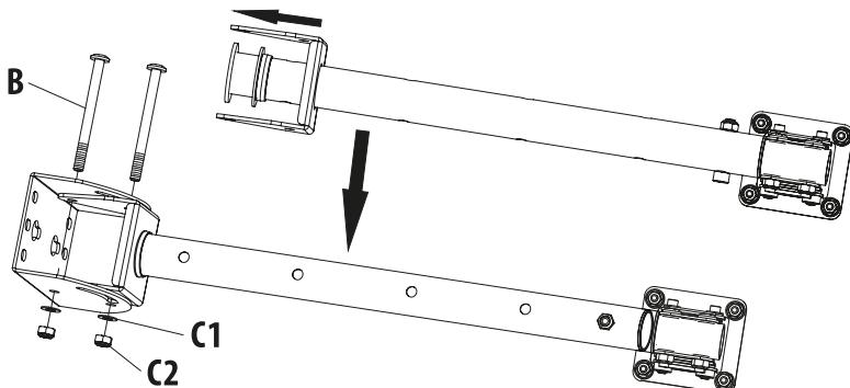
**EN:** Assemble the console head (**M1**) and shaft (**M2**) with the two M8 x 95 axle (**B**) of the accessory. Use the washer (**C1**) and nut (**C2**) in the bag to secure the axle. Position one axle so that it can be adjusted freely to an angle of 45 degrees, while use the hole in the center to secure the other.
