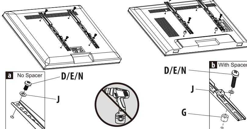
**EN:** Mount the two VESA-compliant mounting rails (**M4**) on the back of the TV. When mounting, use a spacer between the back of the TV and the rail (**G**) if necessary. Use the appropriate screw (**D/E/N**) and washer (**J**) for your TV to mount the rail.
