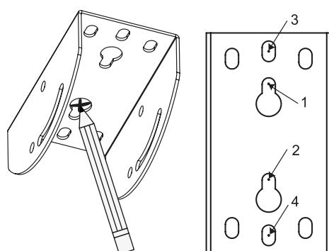
**EN:** After selecting the appropriate load-bearing location for mounting the bracket, place component **(M1)** on the ceiling and use a pen to select at least 4 mounting points. We recommend choosing the holes in the center of the console.
