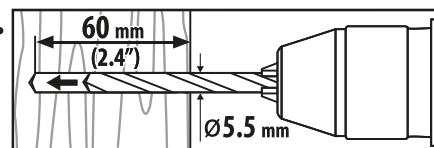
**EN:** Drill 4 holes according to the markings. Use a 5.5 mm diameter drill bit for this operation, with a hole depth of 60 mm!
